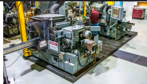
Centerless Grinding Lines
